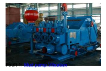
Cause: Pump shaft and motor different heart, impeller imbalance, bearing damage.
